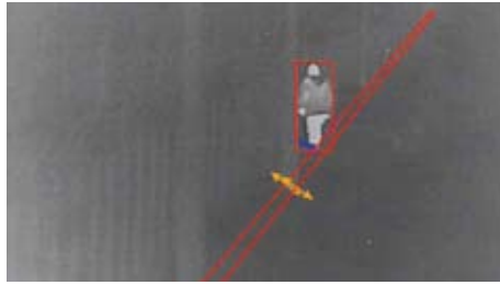
Object Video utilizes algorithms, such as trip wires and areas of interest, to detect objects, and immediately generates useful output such as real-time alerts or triggers for other applications. It works perfectly together with the SR-100 thermal imaging cameras.
