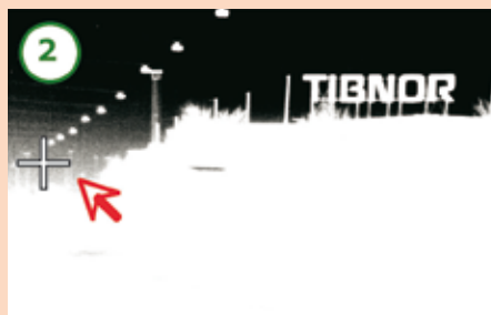
Picture 7: DDE applied - all targets can be observed simultaneously
