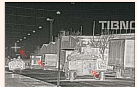
Picture 10: DDE – high & low contrast targets can be observed simultaneously
