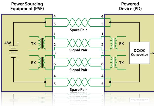
PoE eliminates the need for a separate power source and conduit run for each camera on the network. The only additional cost is for some minor electrical hardware associated with PoE.
