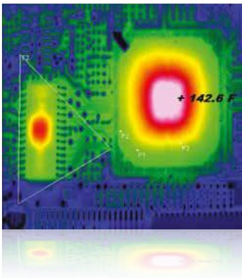
One example of the latter is automated inspection of operating ICs on a circuit board (Figure 1).
