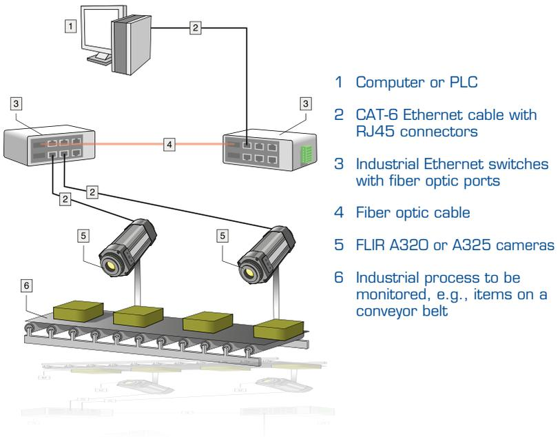
The IR camera's area tools are applied to the thermographic image to check for the minimum allowable temperature of the two parts. If either temperature is below the setpoint (typically, the ambient temperature), then a digital output to a PLC causes an alarm to be sounded and the molding line is halted so the parts can be removed.
