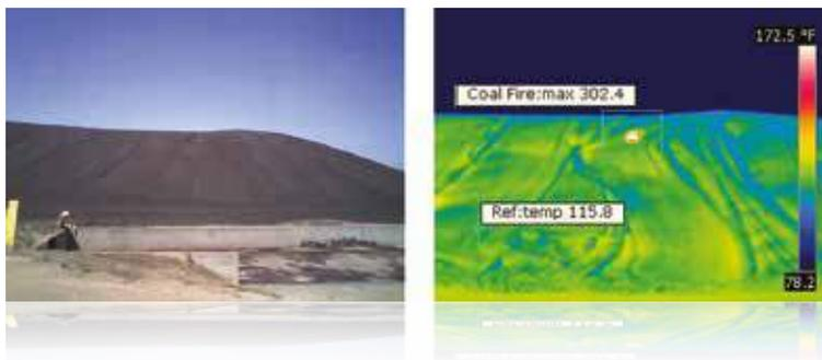
Although self-ignition usually starts within the bottom layers of a stock pile, continuous monitoring of the surface reveals hot spots at an early stage (Figure 8), so measures can be taken to prevent a major fire from breaking out. Large storage yards generally require multiple cameras for total coverage, with the cameras mounted on metal masts above the stock piles. This calls for cameras with housings and other features designed for reliable operation in harsh industrial environments.
