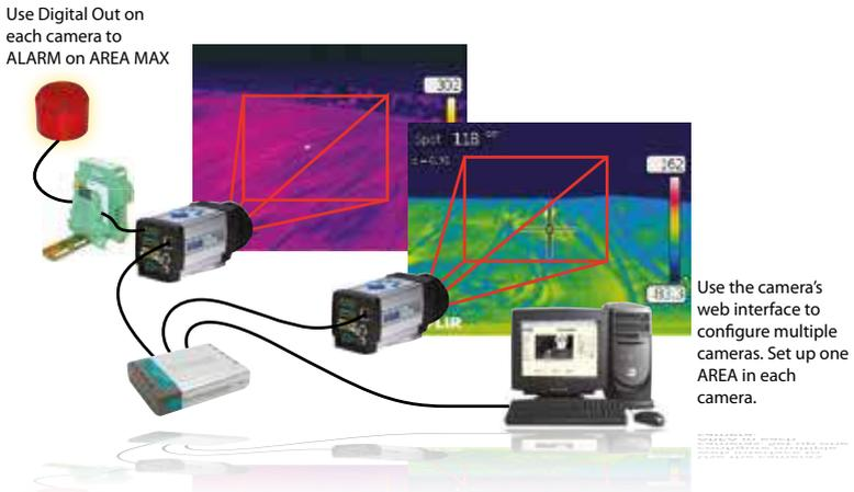
A320 cameras can also be configured to automatically send temperature data and images to a PC via e-mail (SMTP) or ftp protocol whenever the temperature setpoint is reached, thereby creating a record for subsequent review.
