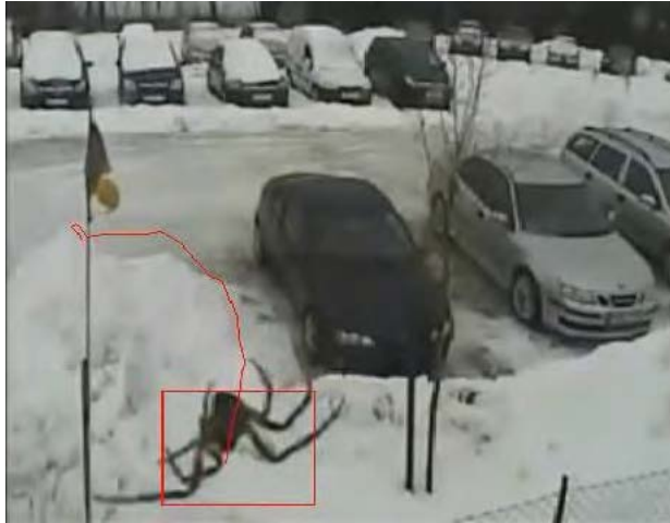
Object Sensitivity 3 – Spider is Detected
