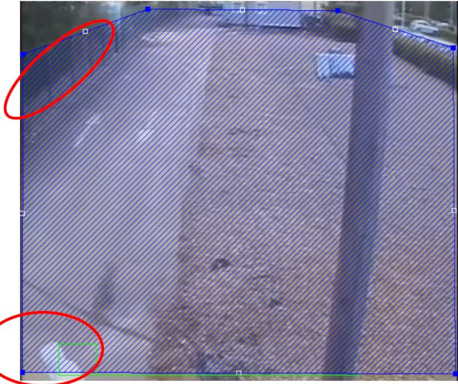
Poor detection area placement
