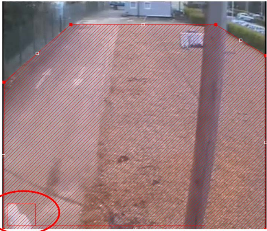
Good detection area placement
