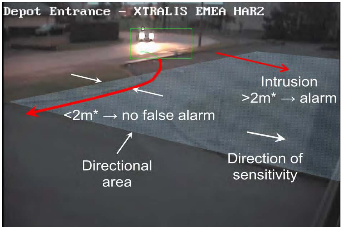
The use of a directional area to filter these false alarms where 2m is set by the minimum distance setting in the advanced configuration
